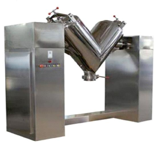
**Genesis V-Shell** Blenders uniformly displace materials for a complete blending of products via the intermeshed action of two inclined cylinders attached together in the form of a "V". This results in precise blending with short mix cycles. Tumble blending is most suited to products of uniform product size and density, and where requirements for fast, thorough cleaning are desirable in sanitary applications.
